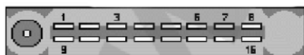
TRIUM ARIA, ARIA® 1-GND 6-Tx 7-Rx 16-VCC 3-R1K to GND 10-R1K to GND
